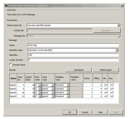
• CANdb specified signals: Allows you to specify a CAN database file that contains message and signal definitions. If you select this option, select a CANdb file. The number of block inputs depends on the number of signals specified in the CANdb file for the selected message.
