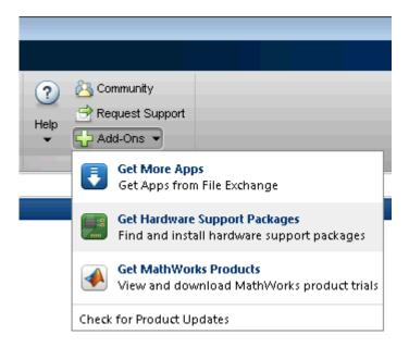
1 The Support Package Installer opens with **Install from Internet** selected. At Support package to install, select PEAK-System CAN Devices.
