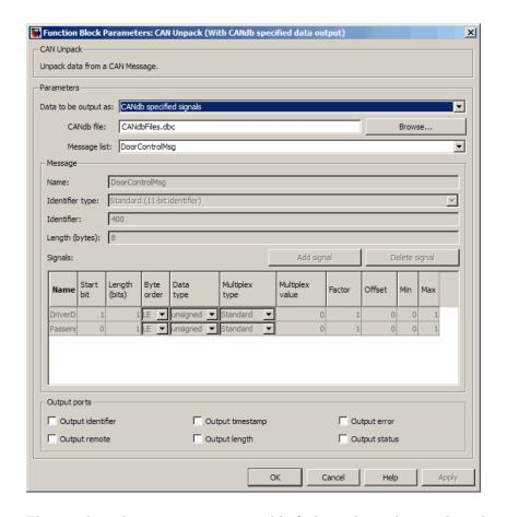
The number of output ports on your block depends on the number of signals specified in the CANdb file. For example, if the selected message in the CANdb file has four signals, your block has four output ports.
