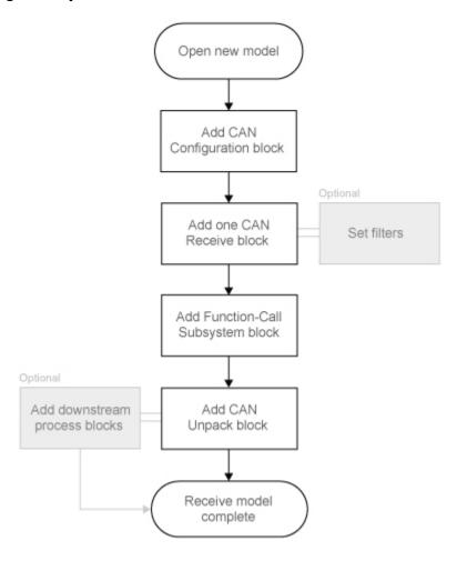
For workflow examples, see "Build CAN Communication Simulink Models" on page 9-11 and the Vehicle Network Toolbox demos.
