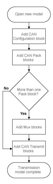
This workflow represents the most common CAN Transmit model. Adjust your model as needed. For more workflow examples, see "Build CAN Communication Simulink Models" on page 9-11 and the Vehicle Network Toolbox demos.
